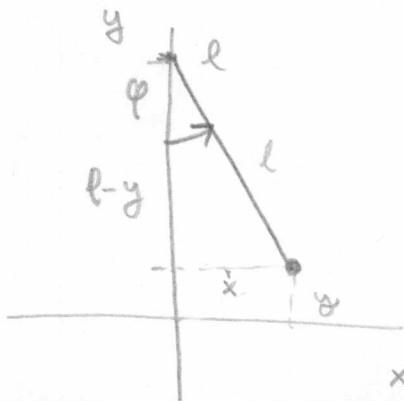
$$x^2 + (y-l)^2 = l^2 \text{ constraint}$$
