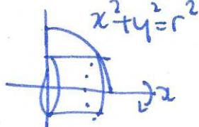
volume of hemisphere: rotate horizontal rectangle about x-axis.
