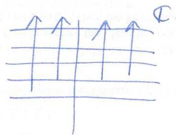
field between two parallel conductors
