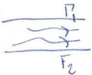
then each curve in  $\partial G$  must be a streamline for the flow (flow can't cross boundary), i.e.  $\psi(x, y) = \text{const}$  on  $\partial G$ .
