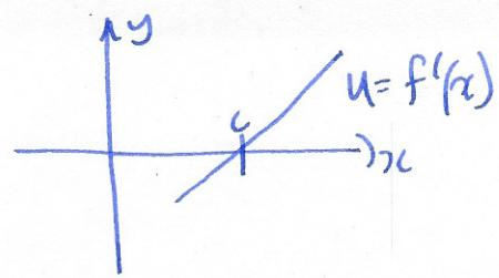
$f'(x)$  goes from negative to positive  $\Rightarrow$  local min.Thus First derivative test If  $f(x)$  is differentiable and  $f'(c) = 0$ then if  $f'(x)$  changes from +ve to -ve at  $c \Rightarrow c$  local max
