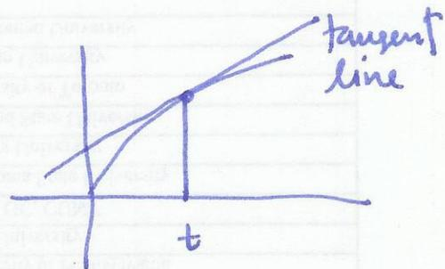
A: speed is slope of tangent line at  $t$ .
