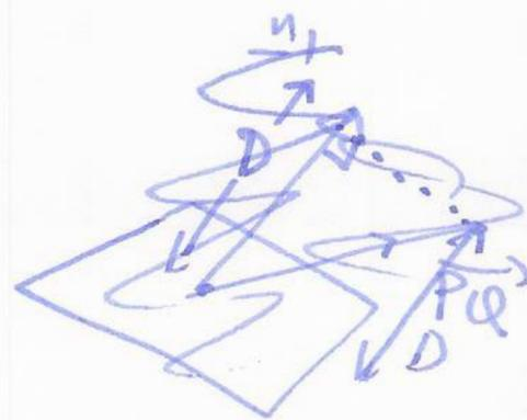
distance from Q to plane =  $\| \text{proj}_{\underline{n}} (\vec{PQ}) \|$
