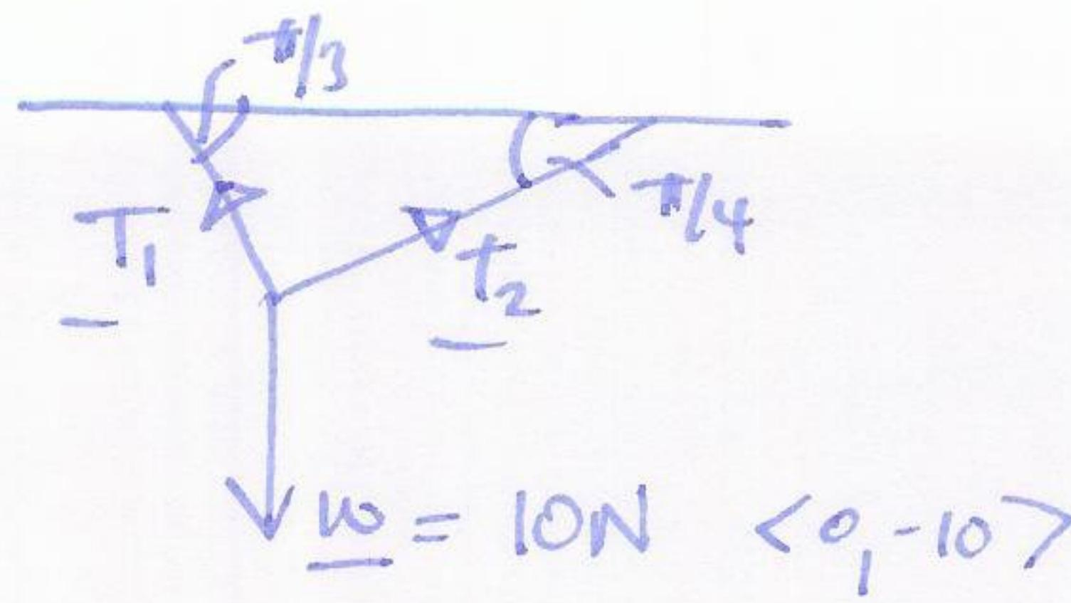
a weight hangs in balance / equilibrium suspended by wires making angles of  $\frac{\pi}{3}$  and  $\frac{\pi}{4}$ . Find the force/tension in each wire.
