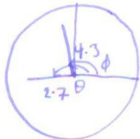
$$\frac{d\phi}{dt} = -2\pi \text{ radians/hour} \quad \frac{d\theta}{dt} = -\frac{2\pi}{12} \text{ radians/hour}$$
